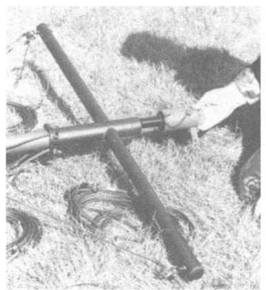
Top crossarm and balun transformer Assembly on mast head.
