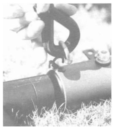
Coaxial cable strain relief fitting on balun transformer.
