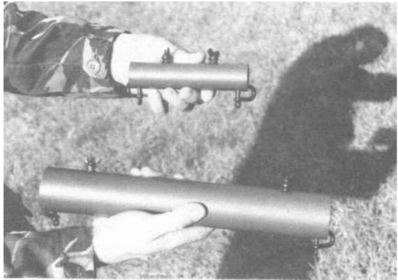
Comparison between CC-104017-3A (100W) & CC-104017-3 (400W) load resistors. The 400W unit is larger.
