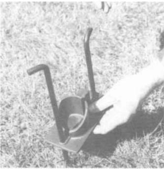
Pinning the mast base to the ground.
